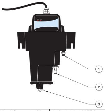
1. Sample Inlet, ¼-28 NPT x ¼-inch Compression fitting2. Drain, ½-inch NPT fitting3. Service Drain
