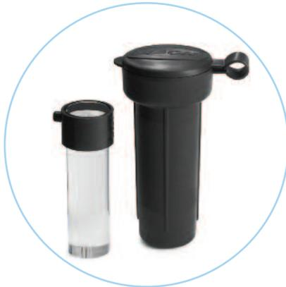
*The Verification Quick Check is a dry method that verifies calibration to below 0.1 NTU (100 mNTU).*
