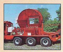
Two hydraulic stabilizing legs and two hydraulic outriggers provide added stability during operation.
