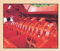
Full hydraulic tub tilt provides safe and easy access to hammermill during routine maintenance.
